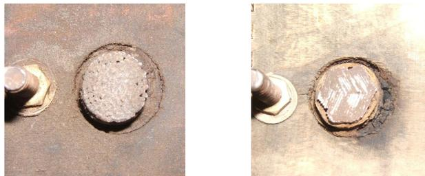
On the left is the more common "bundle of wires" on the right is the laminated construction. The newer coils all seem to be of the laminated construction kind. That includes the KW coils made in the 1950's.
